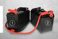
Cross reference the voltage on each battery now they are in parallel – they should both now read a similar voltage.
