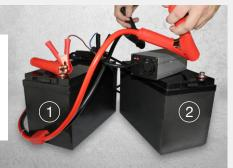
The charger should continue to charge the Lithium battery, bringing it out of safe mode.
